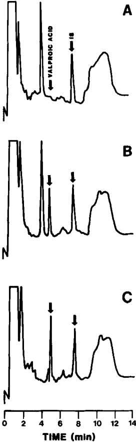
Figure 1. Typical Valproic Acid HPLC Chromatograms. Key: A, 0.0 µg/mL Serum Standard; B, 50.0 µg/mL Serum Standard; and C, Patient Serum Sample (Equivalent to 71.9 µg/mL Serum).
